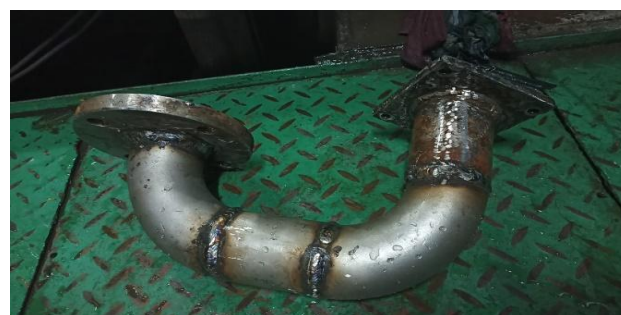
Figure 1: Seawater Cooler Pipe
