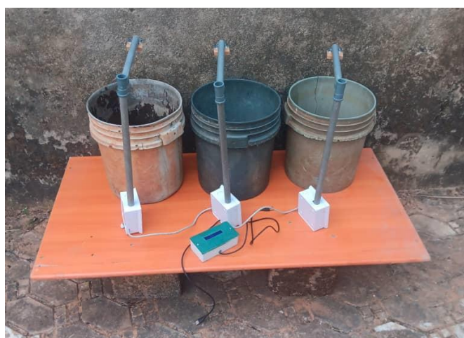
Figure 7.1: Validation and Hardware Implementation of the IoT Based Real Time prototypical Flood Monitoring System for Three communities in Anambra West Nigeria
