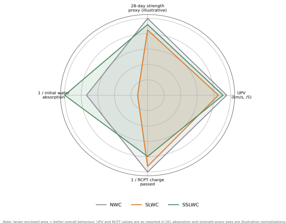
Figure 6: Normalized durability and performance profile of scoria based lightweight concretes versus normal weight control, synthesized from [4]
