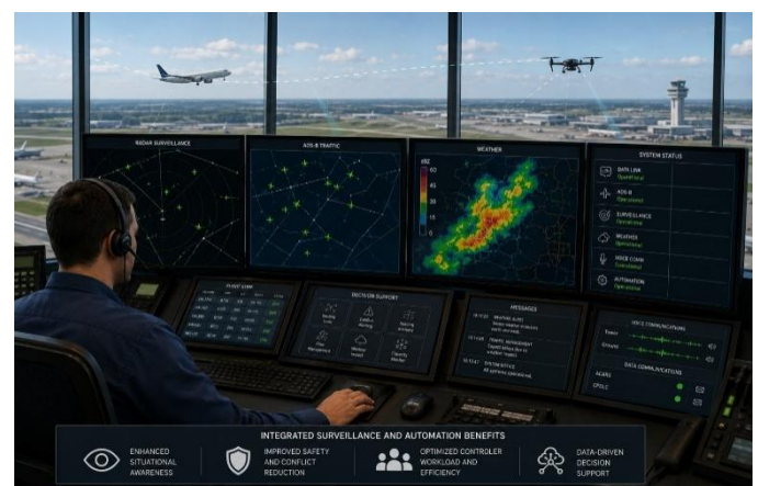
Figure 2: Conceptual illustration of a modern air traffic control workstation integrating radar, ADS-B, weather, communications, and decision-support information to support controller situational awareness
