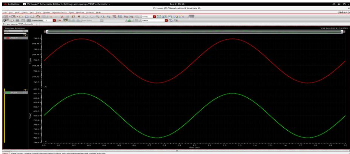
Figure 10: Transient response of operational amplifier
