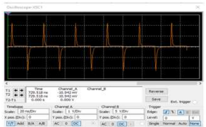
Figure 4: Simulation output of the HPF connected with 74LS04D IC
