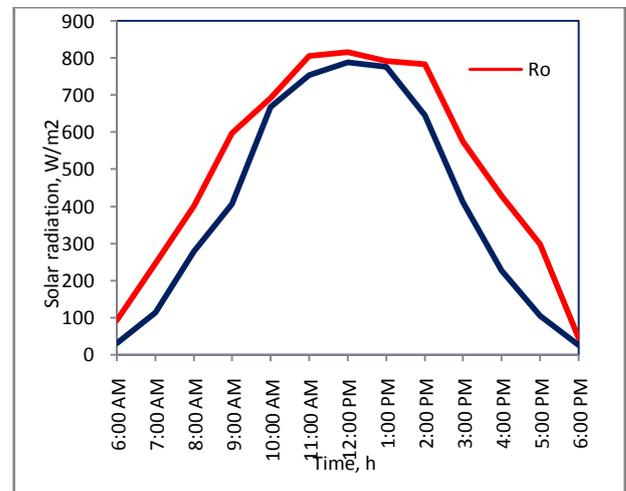
**Figure 5: Distribution of the average solar radiation flux incident outside and inside the solar dryer during the field tests**
