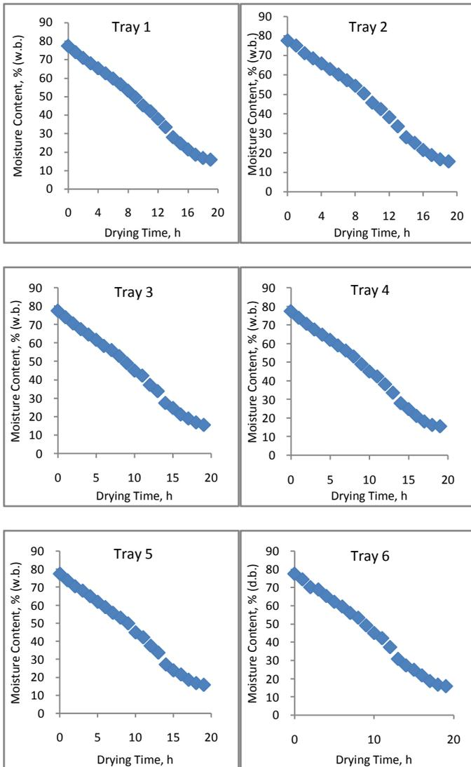
**Figure 8: Changes in the moisture content of grapes (w.b.) with drying time at six different drying trays inside the solar dryer**
