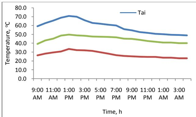
**Figure 6: Indoor, outdoor air temperatures and grape bulk temperature during solar drying process**
