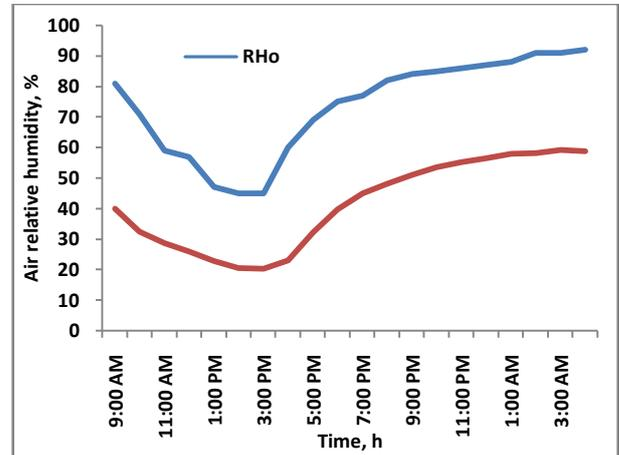
**Figure 7: Indoor, outdoor air relative humidity during solar drying process**
