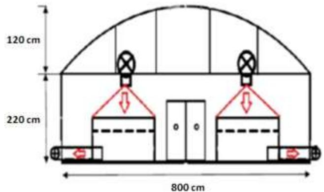
Figure 2: Front view of the dryer frame and bed structure
