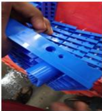
Figure 3: Hole created on side of battery lid
