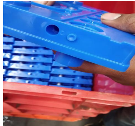
Figure 5: Filler Material fill in hole created after molding process
