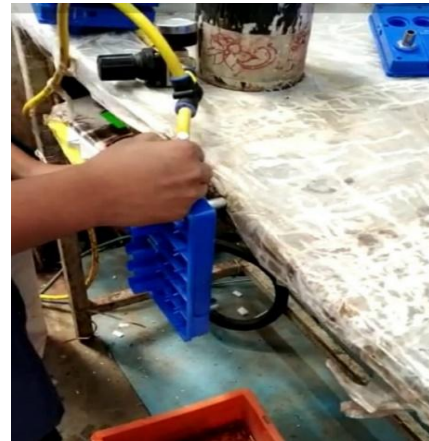
Figure 10: Leakage Marking Manually
