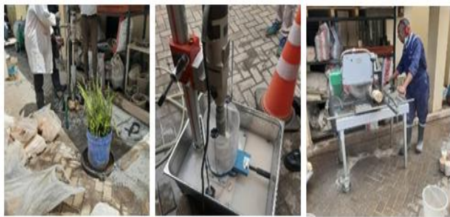
(a) Core drilling (b) Core drilling (c) Grinding to size Figure 6: Rock coring
