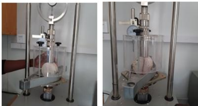
(a) Before failure (b) Post failure Figure 12: Brazilian test setup
