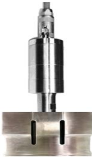
Figure 11: Connection of fabricated slotted block horn with transducer
