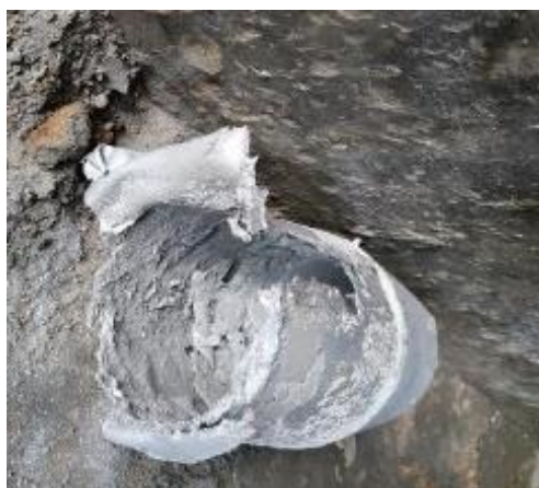
Figure 2: Example of Incomplete Defect
