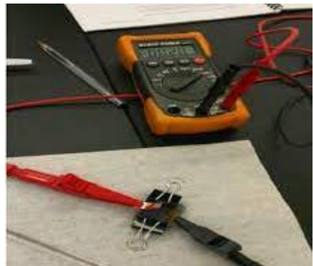
Figure 5: Laboratory prepared Dye solar cell
