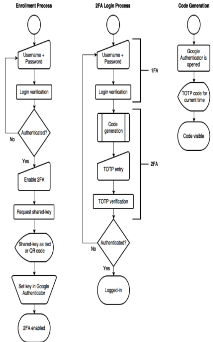
Figure 3: Flow Chart of E-Authentication Login and Code Generation Process
