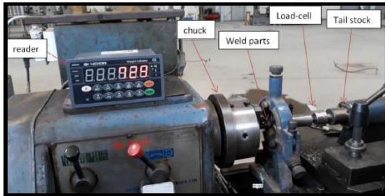
Figure (2): (TAKISAWA) lathe machine that used for rotary friction welding and (load-cell) tying on the tail stock
