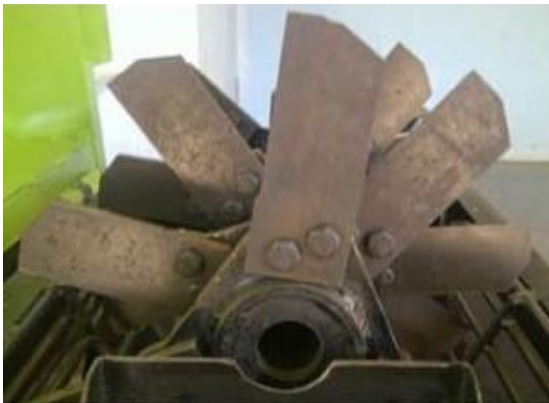
Figure 1: Blade of organic fertilizer chopper
