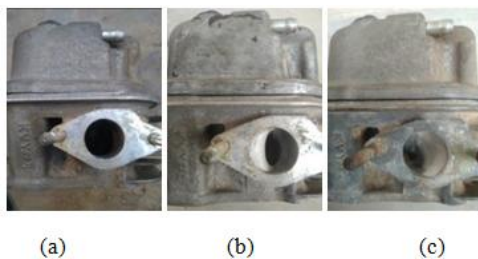
Figure 1: Intake manifold test model (a) tangential port; (b) helical port left; (c) helical port right
