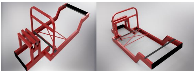
Figure 1: Design of an electric car chassis using Autodesk Inventor professional 2019
