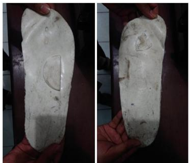
Figure 14: Temperature 75°C, Pressure 150 bar, Talc Composition 10%
