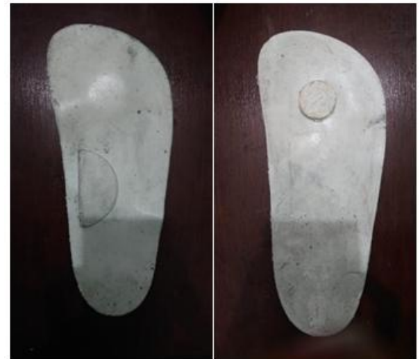
Figure 13: Temperature 75°C, Pressure 150 bar, Talc Composition 20%
