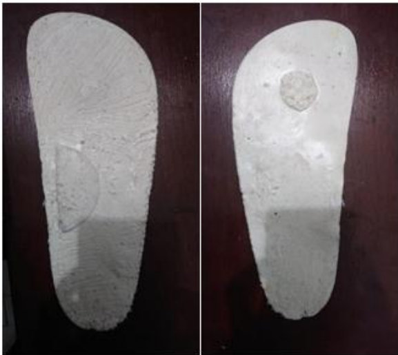
Figure 10: Temperature 100°C, Pressure 150 bar, Talc Composition 20%
