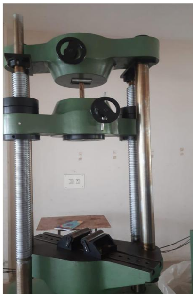
Figure 8: Experimental set up for tensile test
