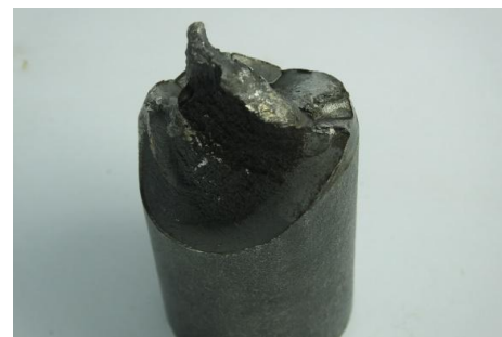
Figure 3: The fault surface is filamentous and forms a 45^\circ
