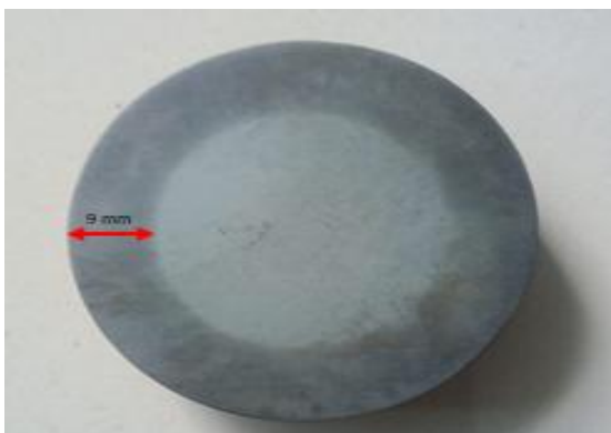
Figure 6: Case hardening thickness
