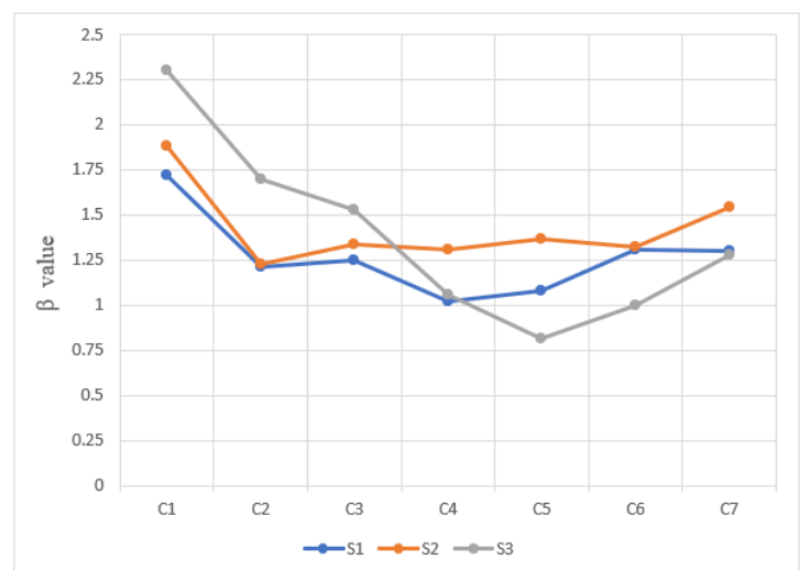
Figure 17: The relation between \beta value and different spans with different columns dimensions
