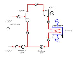
Figure 2: Single flash system in GPP (Valdimarson, 2011)
