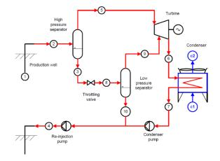
Figure 3: Double flash system in GPP (Valdimarson, 2011)
