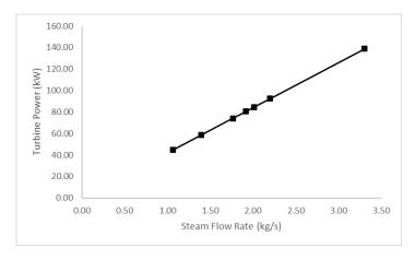
Figure 5: Steam turbine performance curve
