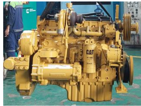
Figure 2: Caterpillar C9 Acert engine after maintenance process
