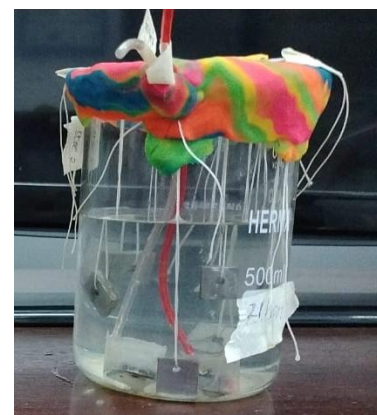
Figure 1: Set up for galvanized steel immersion
