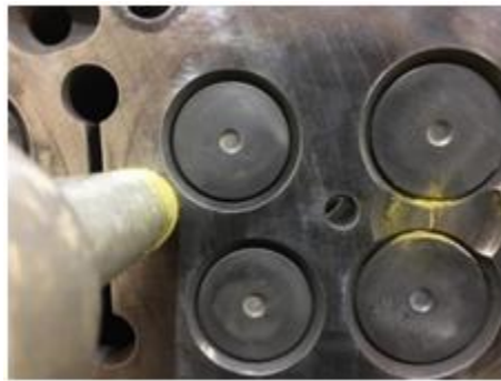
Figure 5: Damage to the cylinder head block
