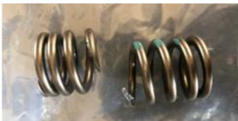
Figure 4: Spring valve damage
