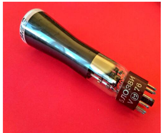
Figure 4: 5LO30I cathode ray tube
