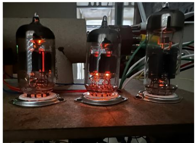
Figure 8: Vacuum tubes inside the oscilloscope in operation
