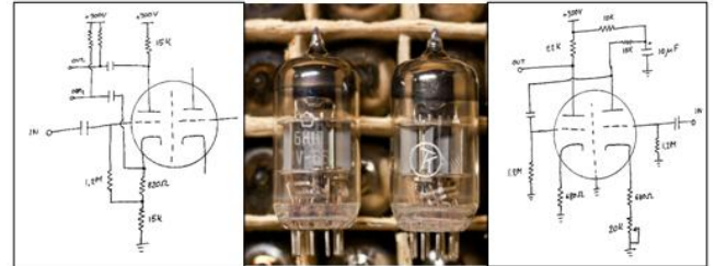
Figure 3: 6N1P vacuum tubes (center) with detection amplifier (left) and input amplifier (right)
