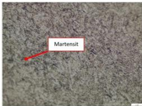
Figure 5: Micro Test Results of pinion gear tooth surface parts
