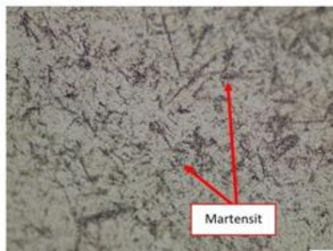
Figure 6: Micro Test Results of pinion gear tooth core parts
