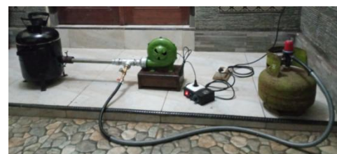
Figure 6: Melting furnace system circuit
