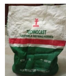
Figure 2: Castable for furnace wall
