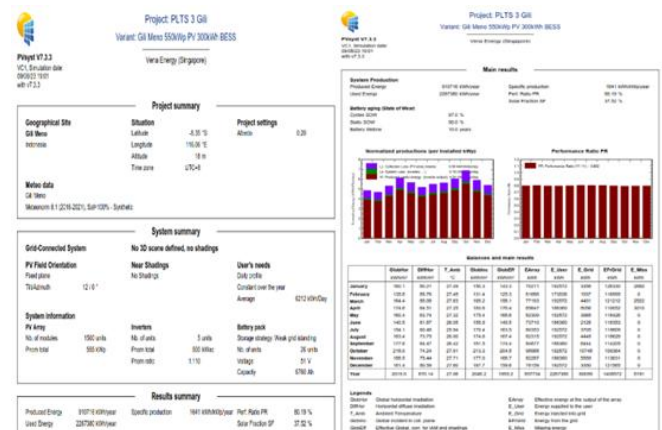
Figure 4: PVsyst Simulation Results for Solar Power Plant with the Addition of Battery in Gili Meno
