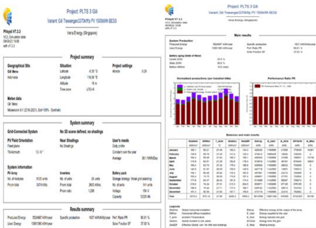
Figure 6: PVsyst Simulation Results for Solar Power Plant with the Addition of Battery in Gili Trawangan
