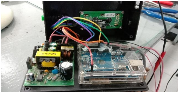
Figure 10: Arduino UNO System Series, Snsor DHT 11 connected with several components on the PCB Board (Casing)
