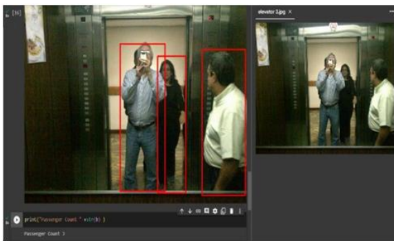
Figure 1: Identified 3 passengers inside elevator
