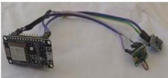
Figure 3: Connection of MAX30100 and MPU-6050 sensor with smart band
