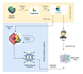
Figure 4: System Diagram Automated Threat Intelligence
