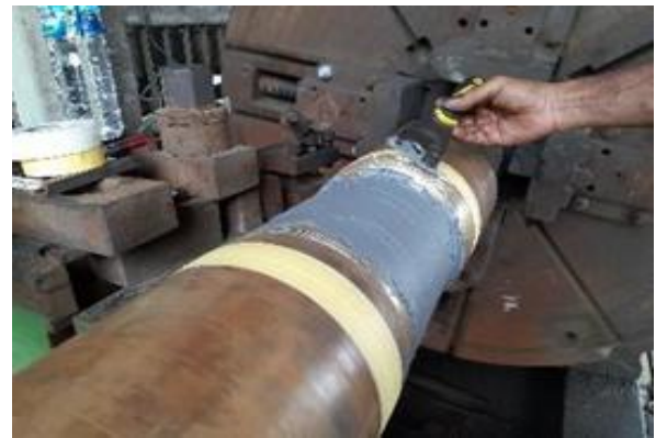
Figure 5: Application of composites to the propeller shaft
