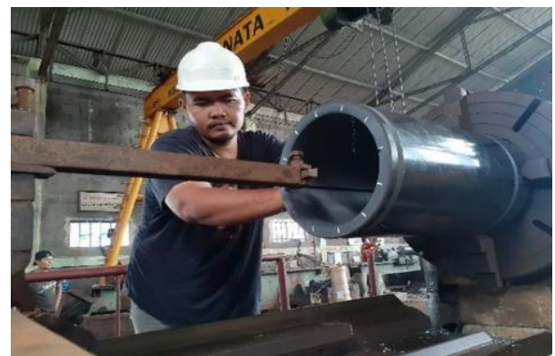
Figure 6: Bearing adjustment using a lathe
