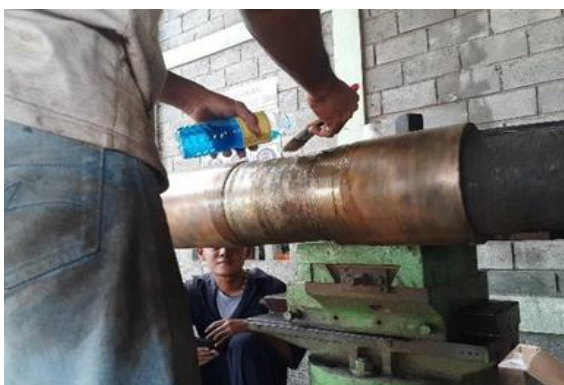
Figure 4: Cleaning rust and remaining paint
