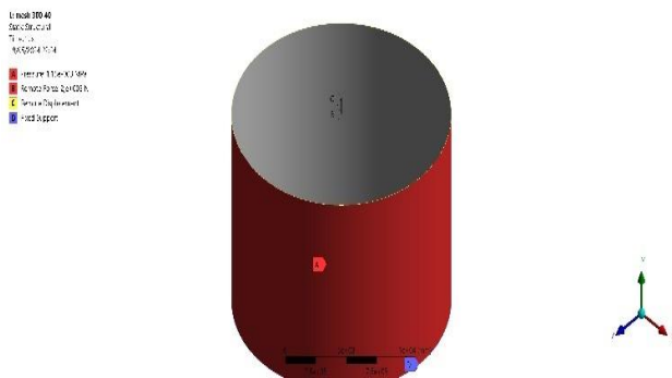
Figure 6: Boundary Conditions and Loading of Cylindrical Tank Using the Analytical Equation of Wind and Roof
