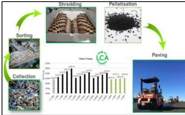
Figure 1: Waste Plastic in Road Construction
