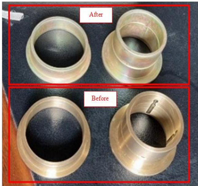
Figure 5: Bushing Differences after the Electroplating Process
