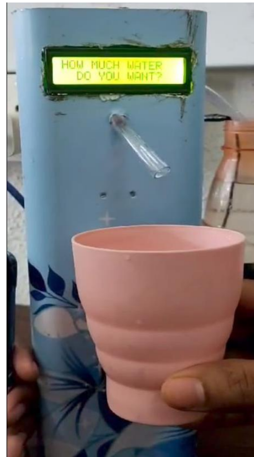
Figure 8: Measures Water To Dispense
