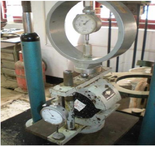
Figure 4.1: Marshall Test in Progress
