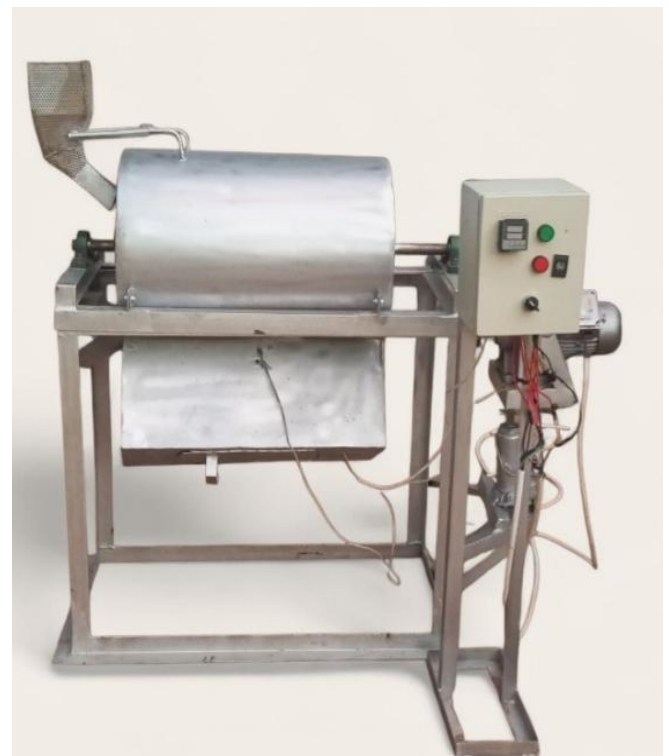
Figure 2: Side view of the cocoa roaster
