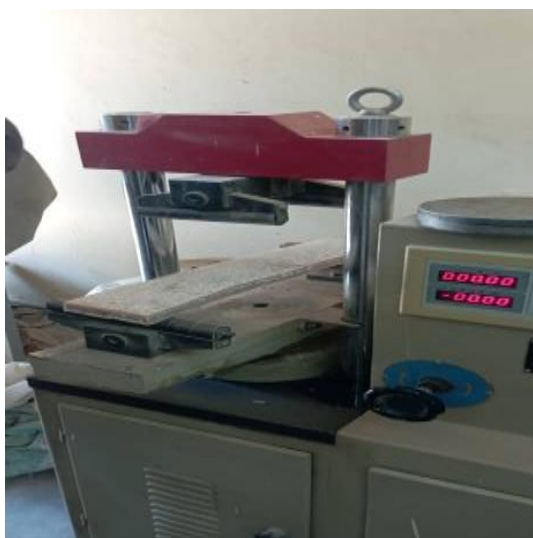
Figure 6: Plywood and fiberglass panels and bending resistance machine
