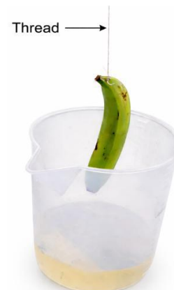
Figure 3: Measure Density Using Water Displacement Method
