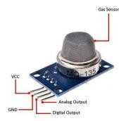
The MQ-135 is a popular gas sensor used for detecting various air pollutants. The MQ-135 is a valuable tool for detecting various gases in the air. The main working of this gas sensor is, it has a semi-conductor material that changes its electrical resistance when exposed to certain gases. The change in resistance is measured and converted into an electrical signal, allowing for the detection and quantification of the presence of gases.
