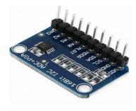
An ADC is like a translator that takes that smooth line and converts it into a series of numbers that a computer can understand and process. In other words, it can also be defined as the device which converts the analog signal into digital signal. In today's digital world, ADCs are crucial components in many electronic devices. They allow us to interface with the real, analog world and process information digitally.
