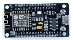
The ESP8266 is a versatile and cost- effective solution for adding Wi-Fi connectivity to various projects. Its affordability, ease of use, and wide range of applications have made it a popular choice in the world of electronics and the Internet of Things.
